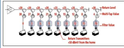
There is a correlation between the tap value and the susceptibility of a subscriber location introducing noise and ingress to the network. The smaller value tap will inherently allow more noise and ingress into the network. By installing a high value RSA on the low value tap, that tap at return band frequencies can
