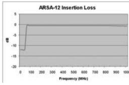
Return step attenuators (RSAs) provide much of the benefit of installing a high pass filter while retaining the ability for two-way operation. RSAs have minimum attenuation at frequencies used for the downstream (50  $\tilde{n}$  1000 MHz) and fixed attenuation at frequencies used for the upstream (5- 42 MHz). RSAs are available in attenuations that range from 3 to 25 dB.
