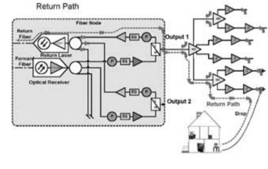
Studies indicate that most sources of ingress occur inside the home. It is therefore important that installation personnel use the proper techniques and are properly equipped so that two-way installations minimize pick up of ingress and noise. This will ensure reliable operation, fewer truck roles, lower maintenance costs and higher customer satisfaction.
