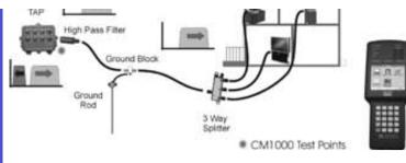
Simply removing the filter and installing a two way set top box or modem exposes the network to ingress the potential problem the filter was intended to eliminate in the first place.
