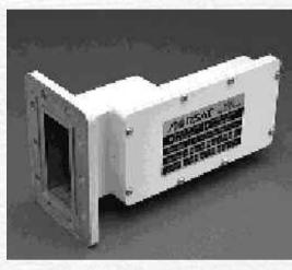
A wideband signal such as an MPEG II television broadcast will require an LNB with low frequency selectivity because the transmitted signal occupies quite a wide bandwidth and the receiver tuning can be wider. A narrow band SCPC radio broadcast uses a very narrow signal and will require a high stability PLL type so that the receiver is able to track the signal.
