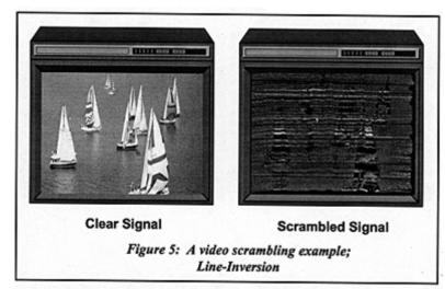
A more sophisticated approach inverts only selected lines within the video frame. This would cause flicker or a superimposed pattern. Such an improvement would be less watchable since it soon causes eye-strain and headache.
