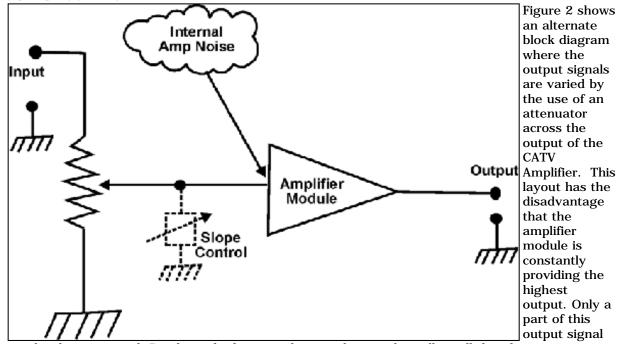
is utilised, as required. Readers who have read our earlier articles will recall that distortion increases very rapidly with output levels. A 5 dB increase in output level will increase the output distortion by 10 dB !
