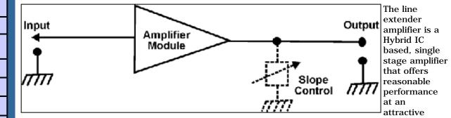
price. Ideally, it should only be used on the branch and last mile paths. It does not offer the lowest level of distortion or noise and hence its use should be avoided on the trunk line. Bridger Amplifiers are usually Hybrid IC based amplifiers that offer high output levels to a branch, for distribution. Some times the Bridge Amplifier; as a module; is housed within the trunk amplifier enclosure.
