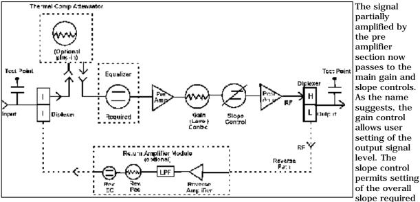
by the system. While some products maintain fixed pads for specific, plug-in gain and slope control values, others offer a variable potentiometer for more versatile, on site control. The advantages and disadvantages of fixed pads versus potentiometers is elaborated a little later.
