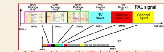
Fig. 1: Number of channels within 8 MHz bandwidth and different types of modulation. DVB-C uses QAM modulation and allows the largest number of channels per 8 MHz.
