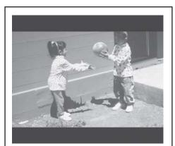
Fig 2b: A 16x9 Movie Reduced To A 4x3 'Letterbox' Picture
