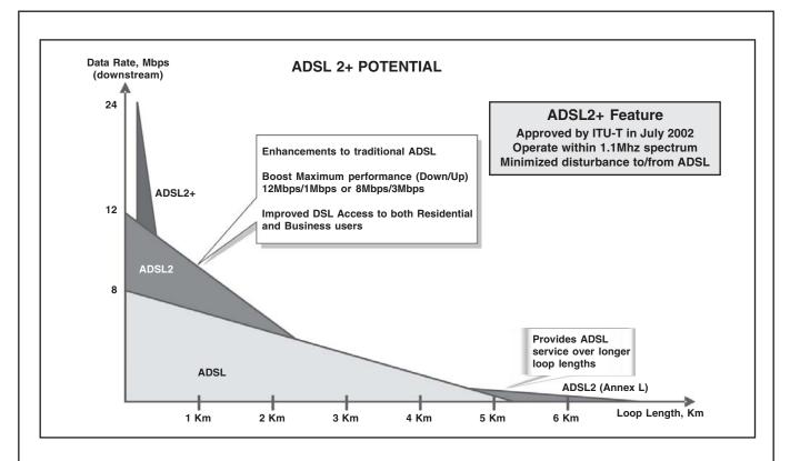
The latest standard ADSL2+ can deliver up to 24Mbps down stream compared to 8 Mbps by ADSL depending on the distance from DSLAM(Digital Subscriber Line Access Multiplier) kept in the telephone exchange.
