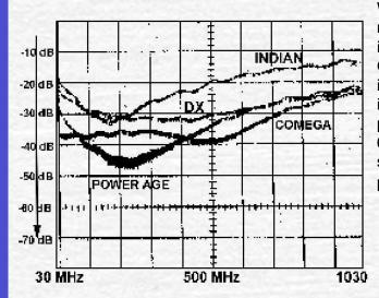
While most good quality locally manufactured passives provide an isolation of 18 dB to 20 dB upto 1 GHz, even this level of performance is inadequate for large networks. It was interesting to measure that Comega passives offered an isolation of upto 60 dB at high frequencies. By any standards, this is exceptional performance.
