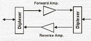
The few networks that utilised the reverse paths did so for relay of one channel. These users soon realised that the frequency band below 20 MHz was almost unusable due to the high amount of noise. This concern remains even today.
