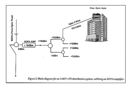
Even if 8 fibre optic trunks are generated, with the use of additional splitters as indicated in Figure 2, each of the 8 fibre optic trunks will have an output of 9 dBm.
